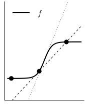
Dotted line is tangent to f where f attains its Lipschitz constant: slope K. The dashed line is the steepest line that intersects any pair of observations: slope  $\hat{K} \leq K$ .
