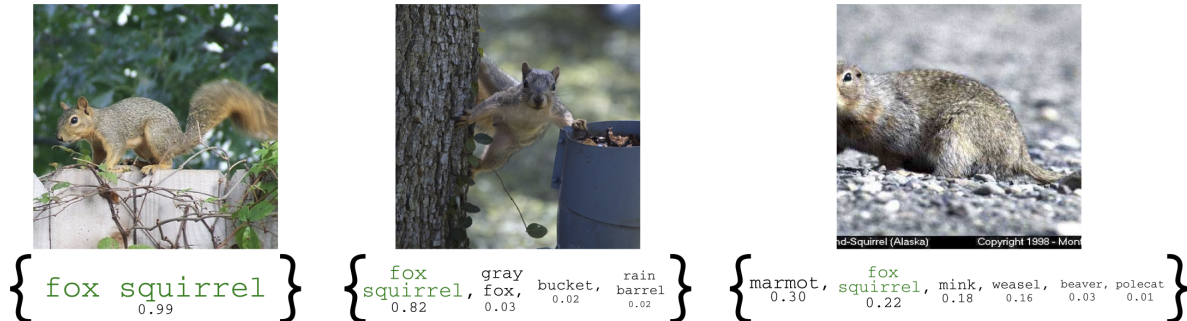
Figure 7: Examples of RAPS, which is conformal prediction with a regularized version of the cumulative likelihood score. The true label in each case is “fox squirrel”, and we can see that the prediction sets adapt appropriately in size to the hardness of the classification task. Credit: Angelopoulos et al. (2021).
