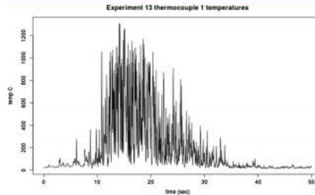
Figure 3. The temperatures ( $^{\circ}\text{C}$ ) recorded at thermocouple 1. There are 25,001 measurements in all
