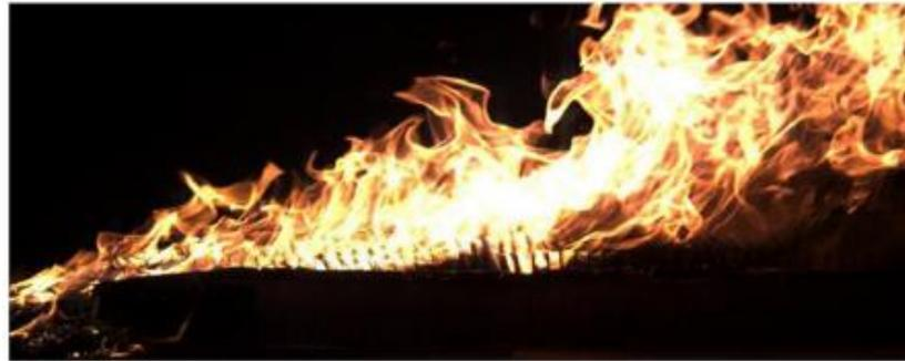
Figure 2. This photo was taken from the side of the testbed. The wind is blowing from the left, and the flames are moving to the right. Some tiles are still standing
