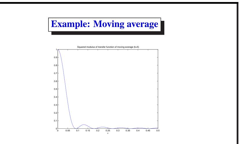
This is a *low-pass filter*: It preserves low frequencies and diminishes high frequencies. It is often used to estimate a monotonic trend component of a series.
