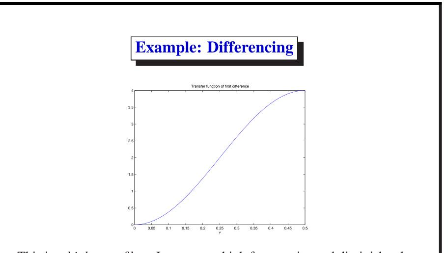
This is a *high-pass filter*: It preserves high frequencies and diminishes low frequencies. It is often used to eliminate a trend component of a series.
