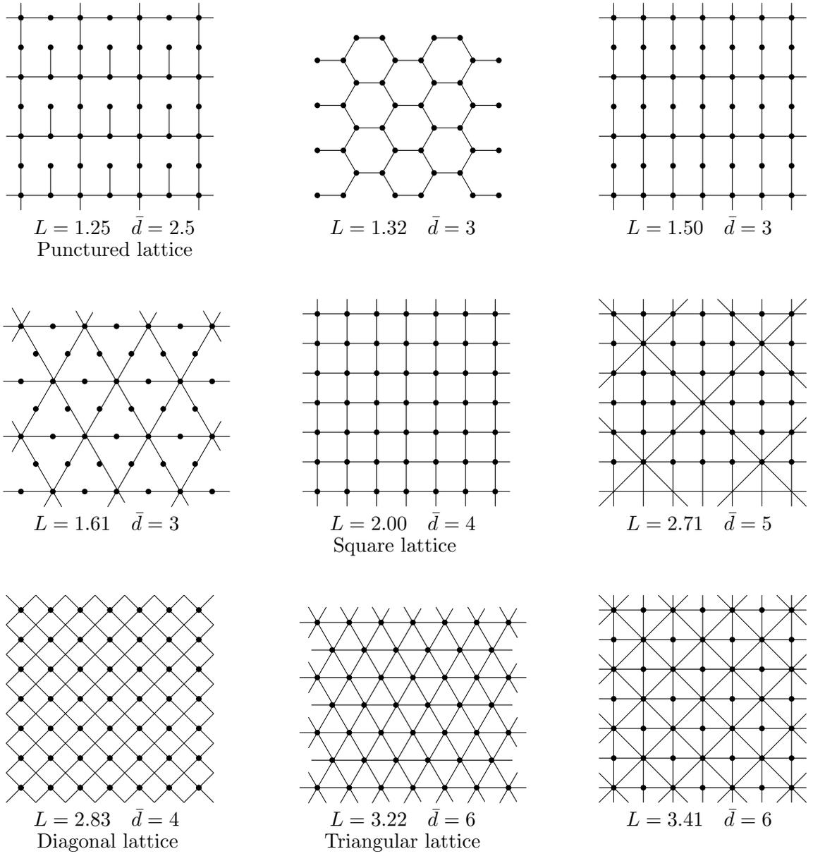
**Figure 4. Variant square, triangular and hexagonal lattices.**
