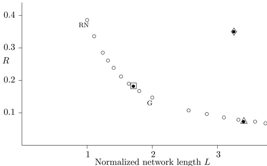
**Figure 7.** The normalized network length  $L$  and the route length efficiency statistic  $R$  for certain networks on random points. The  $\circ$  show the beta-skeleton family, with RN the relative neighborhood graph and G the Gabriel graph. The  $\bullet$  are special models:  $\triangle$  shows the Delaunay triangulation,  $\square$  shows the network  $\mathcal{G}_2$  from section 2.4, and  $\diamond$  shows the Hammersley network.
