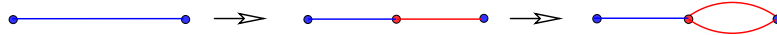
Fig. 3.4. The first is a series step: a road in the current network is replaced by two roads that run one after the other along the same path. The second is a parallel step: A road is replaced by two, each of which runs from the same starting to the same ending points as the current road.
