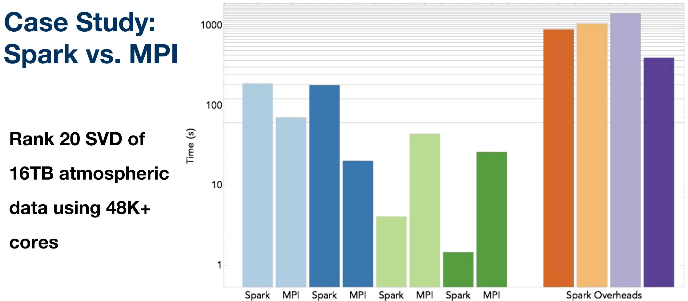
Parallel HDFS Read Gram Matrix Vector Product Distributed A\*V Local SVD A+V Task Start Delay Scheduler Delay Task Overheads Time Waiting Until Stage End
