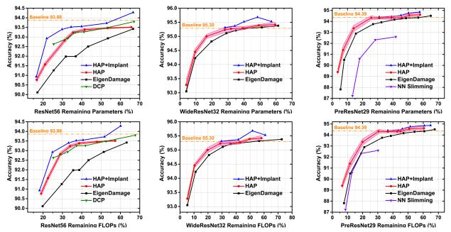
**Figure 2:** Comparison of accuracy with different pruning ratios among HAP+IMPLANT, HAP, NN Slimming, EigenDamage, and DCP, on the CIFAR-10 dataset, for ResNet56, WideResNet32, and PreResNet29. (Top) Remaining parameters in the network after pruning is used for x-axis. (Bottom) Remaining FLOPs in the network after pruning is used for x-axis. HAP consistently outperforms EigenDamage and NN Slimming, and HAP+IMPLANT boosts performance for moderate pruning ratios and surpasses DCP.
