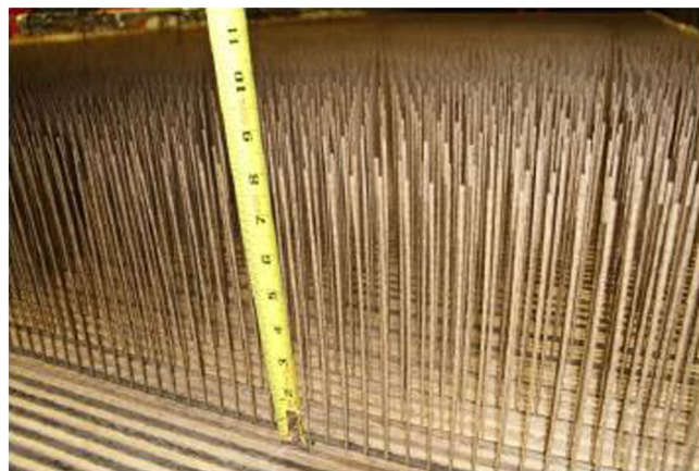
Figure 1. The combs of tines are laid out regularly along a straight testbed
